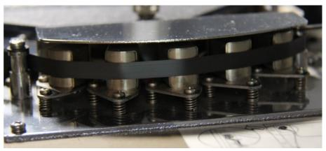
The logic of a tape delay is that the farther the pick-up head is located from the write head, the longer the delay time is. So the first head will have a short delay time, second head will have a medium time and the third head is the one with the longest delay time. This kind of structure is also known as "multi-tap delay". The combinations offered by the MODE selector are:
