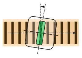
and the head isn't able to erase the tape completely, not only part of the original audio remains on the tape but it is also slightly altered because of the BIAS waveform that alters the tape content the wrong way.
