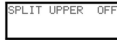
A display like this indicates that there's no split configured for the upper manual, and the button LED n. 8 will blink, indicating that by pressing that button the SPLIT can be activated on the upper manual.
