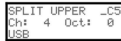
The first line shows a blinking cursor indicating that the split point can be changed by using the rotary encoder. Of course, the split range goes from MIDI Note n. 36 (C3) to Note n. 96 (C8) which is the total range of a 61 note keyboard. Everything below the split point is the split zone that sends notes on the selected split channel, transposed by the selected octave and towards the selected combination of MIDI Output ports.
