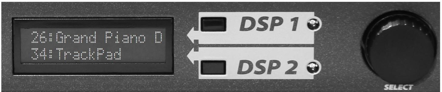
To recall a preset on DSP 1, make sure its LED is illuminated then turn the encoder to browse the preset list. At this point you'll notice that the LED starts flashing, this indicates that you're browsing presets but you still haven't confirmed which one you wish to recall. Once you have found the preset you like, press the corresponding DSP 1 button. If you wish to abort your research and stop the LED from flashing, press the other DSP button.
