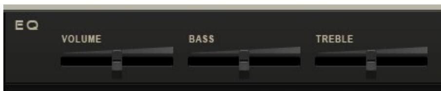
The volume slider is located, within the sound chain, between the output of the instrument and the input of FX1. This is a very important factor because can influence the behaviour of effects based on the input signal's amplitude like the Auto Wah and the Overdrive. For instance, if you are playing a rock organ patch and you want more drive, turn the volume up.
