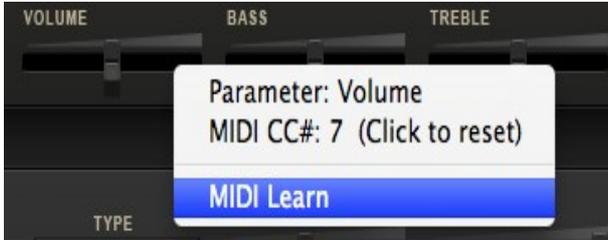
Right-click on a control. A menu should pop-up where the mouse pointer is located. The first line in the menu shows the parameter name. The second line shows the CC number currently assigned. If you click on this menu item, the CC is unassigned. If no CC is
