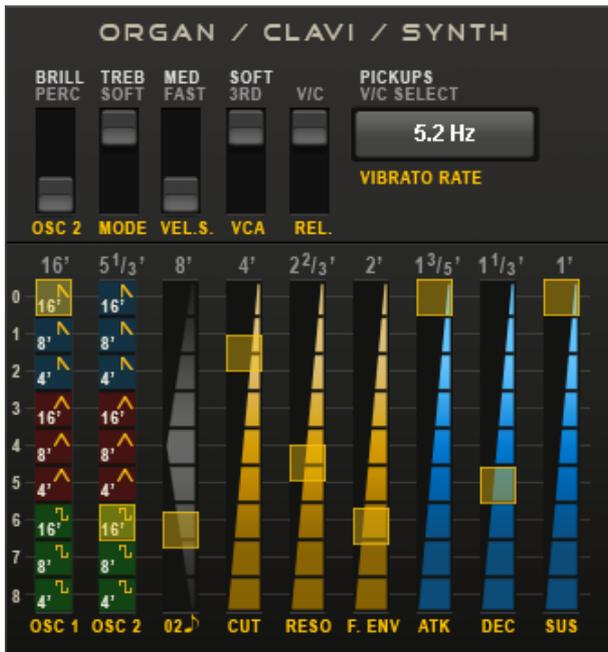
Key Performer also features a built-in 32-voice polyphonic VA synthesizer in subtractive synthesis with two bandlimited alias-free oscillators and a 24 dB resonant low-pass filter.
